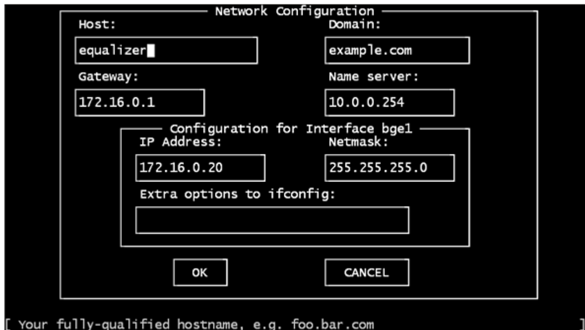
Figure 17 Equalizer Configuration Utility: Network Configuration
